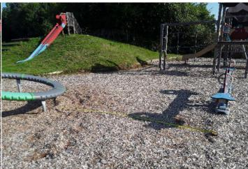
**Finding:** The falling space overlaps the free space between **Action:** Monitor - No remedial work recommended the item and the supernova in contravention of the requirements of BS EN 1176:2017 Part 1
