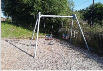
Finding: BS EN 1176 Part 2: Annex A makes a recommendation that fences or enclosures should be upto 1.50m from the edges of the swing seat to the sides, and subject to risk assessment, from the edge of the impact area. This is however, a low risk finding and no remedial action is recommended.
